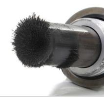
Real-time ferrous wear detection – discover machinery failures faster
